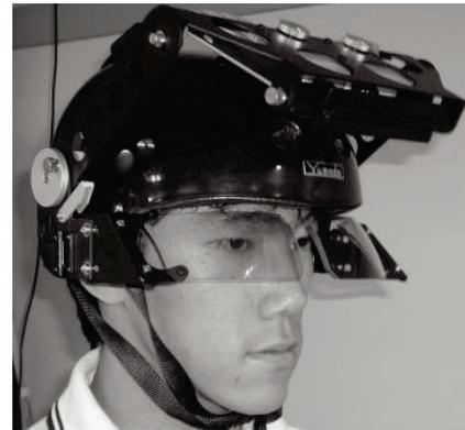
Figure 2. A stereo prototype of HHMPD
