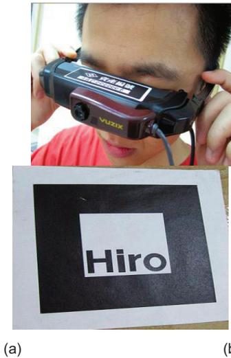
Figure 4. Components for AR visualization (a) HMD and the camera attached; (b) AR pattern
