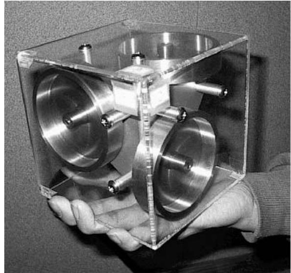
Fig.1 Developed Torque feedback device GyroCube
