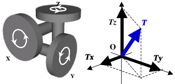
Fig.2 Addition of component angular momentum vectors
