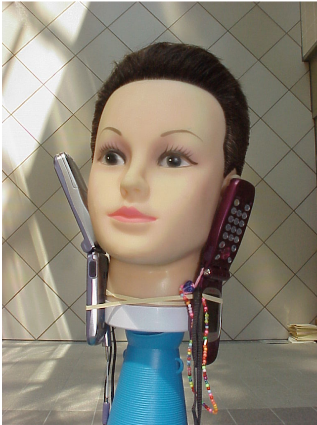
Fig. 9: “Poor person’s mobile stereotelephony:” two mobile phones deployed as a microphone array attached to a dummy head simultaneously calling a dual voice line (like that provided by ISDN) realizes wireless (if still low-fidelity) binaural telepresence.
