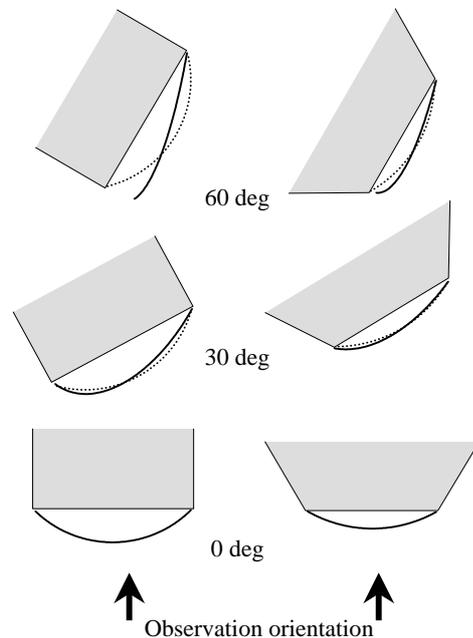
Fig.3 Distortion caused by depth approximation
