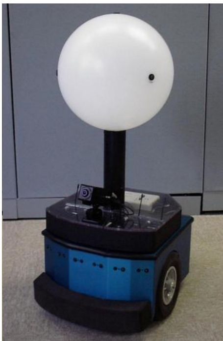
Fig. 2: “Hero” Labo-3 hearing telerobot: operable in piloted and autonomous (automatic obstacle avoidance) modes, with cyclopean (one-eyed) camera and quadraphonic tetrahedral microphone array, shown along with a Java3D model used in simulations.
