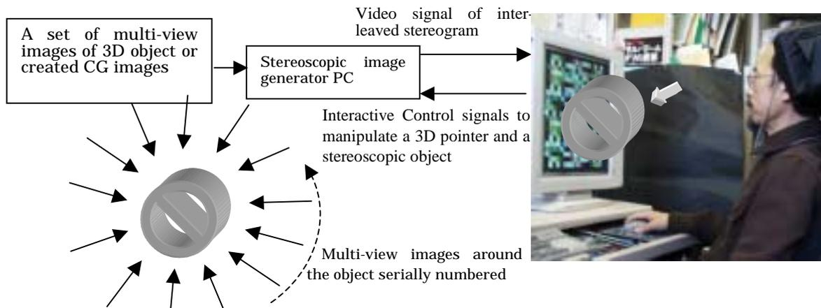
**Fig.1** A diagram of the Interactive multi-view autostereoscopic display system, and a photo and synthesized images showing a figure of viewing a stereoscopic image on the display
