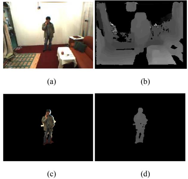
Fig 4. Extraction 3D information of the user. (a) Captured live image (b) Disparity image of the live image (c) The segmented user (d) The disparity image of the segmented user
