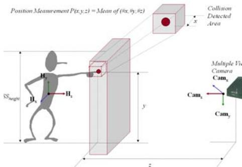
Fig 3. Position measurement of SpaceSensor.
