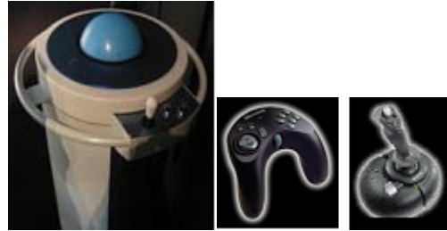
Fig. 19 Standard Interaction devices to use with CyberDomes: Trackball for Big Domes and joysticks for small domes.
