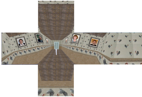
Figure 2. Exploded view of the display. Facing forward the subject viewed a hallway that pitched up and down about an axis that passed through their ears. A bar was displayed in front of the subject that could be adjusted through the use of a gamepad. See also Figure 3.
