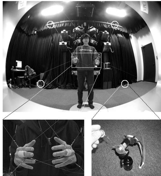
Figure 3 A snapshot of whole system that integrated the SPIDA-H interface into D-vision. User's each hand is connected to 4 strings and motors for force feedback. String-based structure is quite safe, and is less restrictive at user's full body movements.
