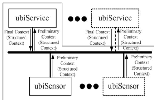
Fig. 2. ubi-UCAM architecture; ubiSensor and ubiService
