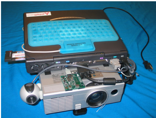
Figure 1 A projector-camera pair. The camera is attached to the projector and the pair is calibrated. The unit depicted is an example of a context-aware unit, which besides camera and projector also consists of a laptop (computing), a tilt sensor and wireless LAN.
