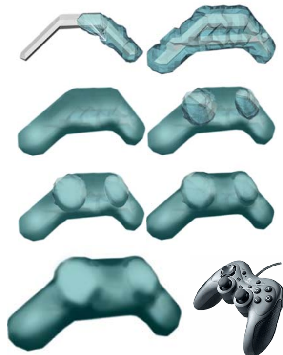
Fig. 8 usage scenario for modeling a game pad (from top left, every image shows the continuous process of form development targeting the final image of bottom right)
