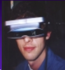
MR Laboratory's COASTAR HMD (Co-Optical Axis See-Through Augmented Reality) Parallax-free video see-through HMD
