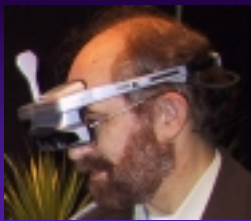
MR Laboratory's COASTAR HMD (Co-Optical Axis See-Through Augmented Reality) Parallax-free video see-through HMD
