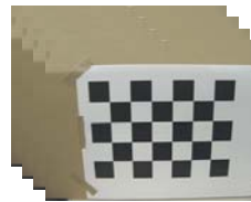
Multiple Images of Checker Pattern Board at Arbitrary Pose
