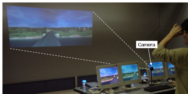
Fig. 3 Basic configuration of image warping and blending system. The center camera is used for generation of warping parameter and blending mask.
