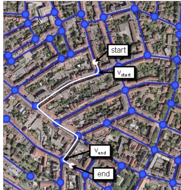
Figure 2: Schematic view of a camera path in the representing road network. The road network is colored blue, while the white shows the calculated camera path.
