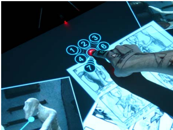
Fig. 4: Laser based touch input.
