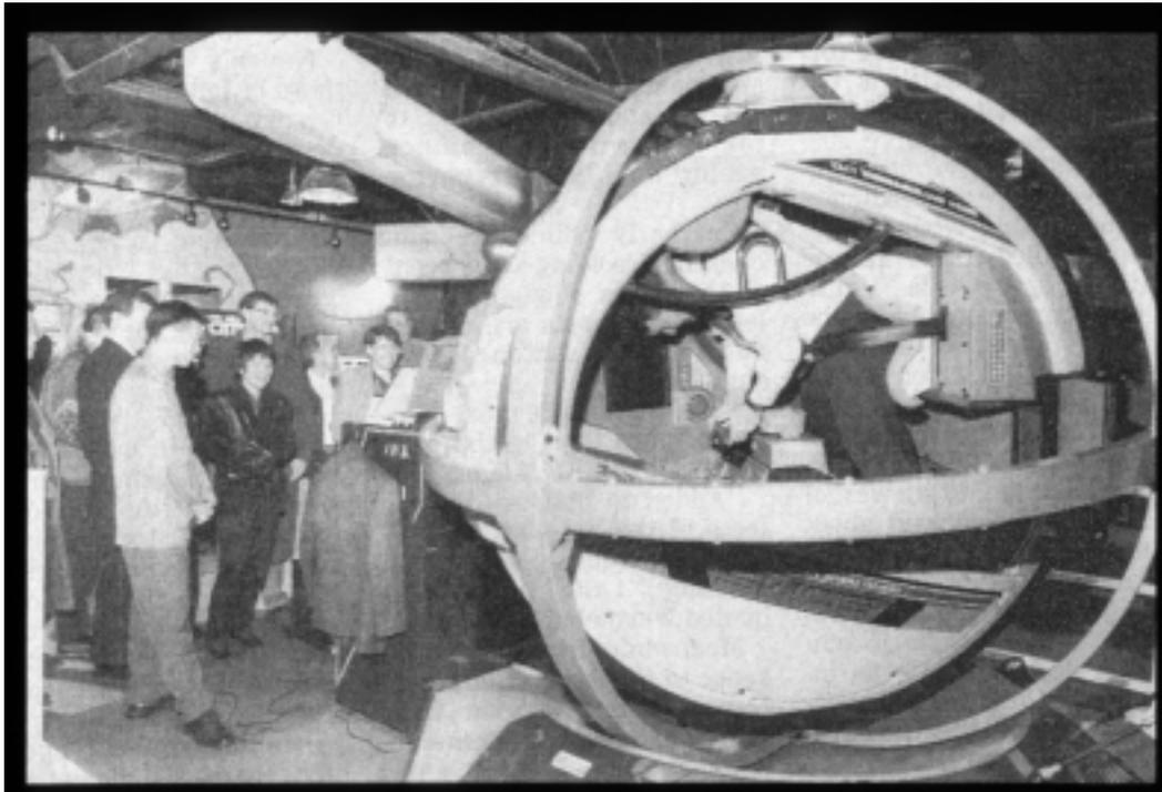
Fig. 3: R360 (SEGA): jet fighter simulator with gimbals providing three rotational degrees of freedom
