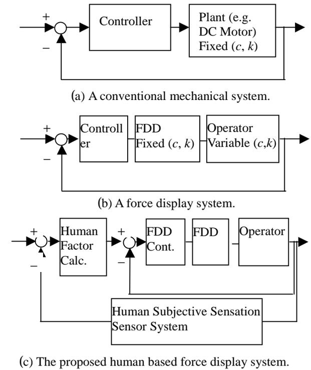
Fig. 1: Control loop structure.
