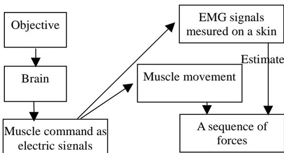
Fig. 8: Flow of signals for straining muscles and the estimation of force sequences by EMG signals.
